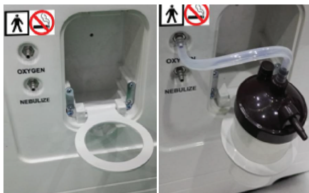
Figure 5 Connection of the Humidifier Bottle diagram
