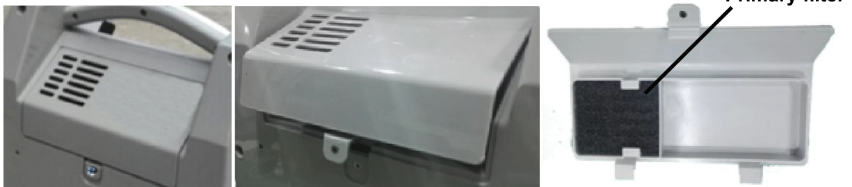
Figure 9 Primary Filter Take Out
