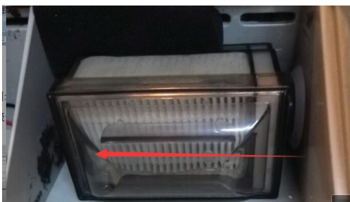
Figure 10 Air Inlet Filter take out
